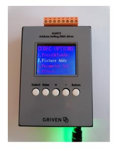
1. Press the "Select" key and choose the option "2. Fixture Addr." Press the "OK" keys to confirm.
