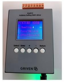
5. Using the + and - keys, select the number of DMX channels each pixel uses.
