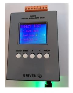
5. MANU GRAY (Automatically Gradual Gray Fade IN/ Fade Out) Using the + and - keys, change current colour. Press "Enter" button key to go to the next option. Using the + and - keys, change gray value. Press the "Select" button to go to return to effect number 1. Press the "Return" key to return to the main screen.
