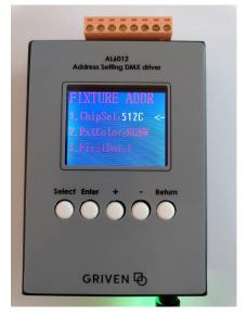
2. Select the chipset to be used using the + and - keys. Here we use 512C for example.
