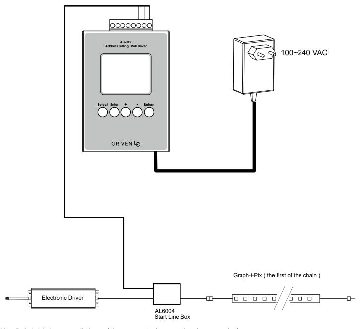
Key Point :Make sure all the cable connected properly, shows as below.
