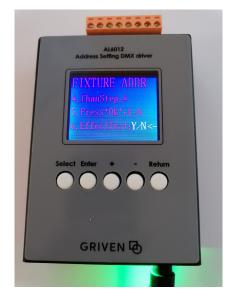
9. Press the "Enter" key to access test light effects.
