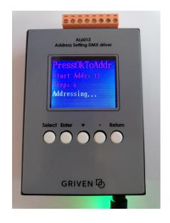
Fast addressing using the last parameters used in option 2. Fixture Addr.
