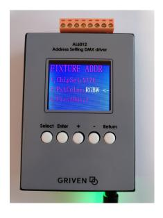
Select the pixel color be used using the + and - keys. Available W, RG (DW), RGB, RGBW. Here we use RGBW for example. Press the "Select" button to go to the next option.
